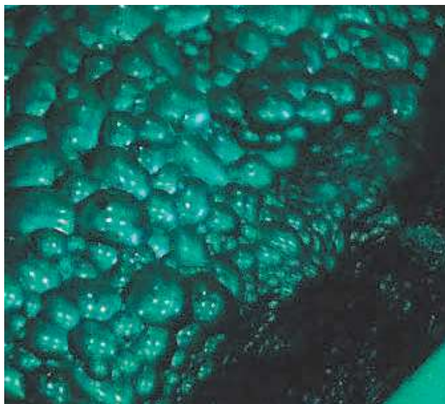
■ Froth flotation as a process to collect certain metals from mineral ores
